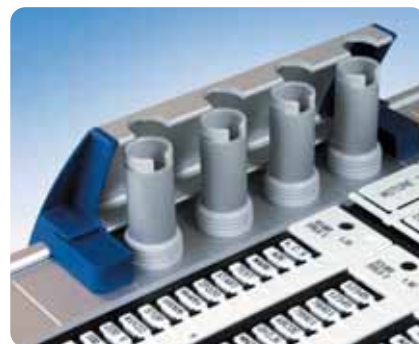
After printing, the pen is returned to a special airtight holder within the plotter.
